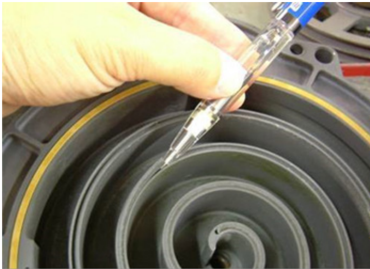
Figure 33: HP Tip Seal Removal
