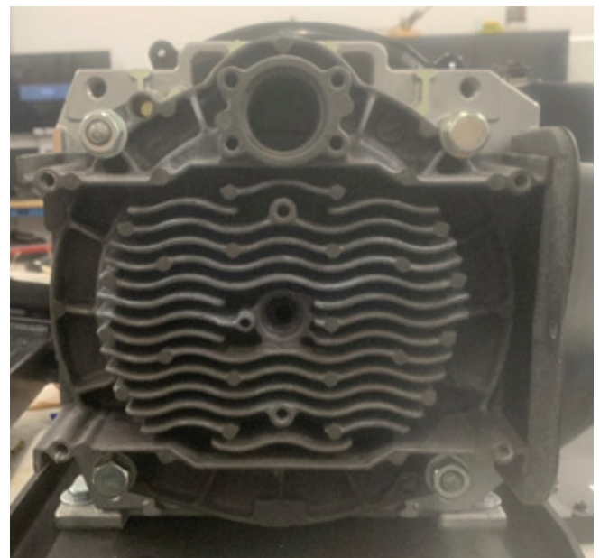
Figure 52: Fixed scroll with fins exposed
