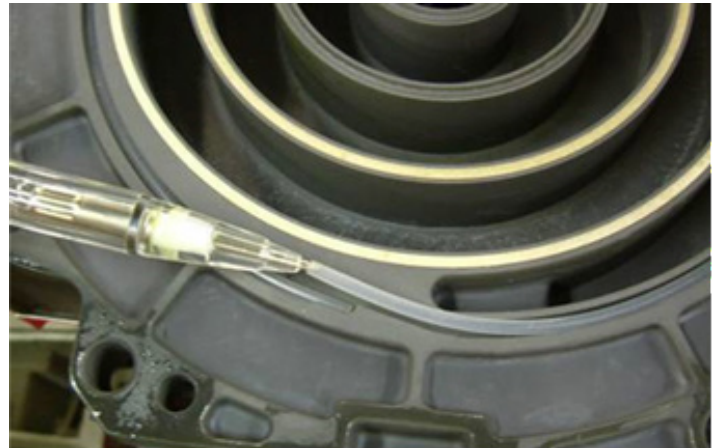
Figure 35: Back-up Tube Removal
