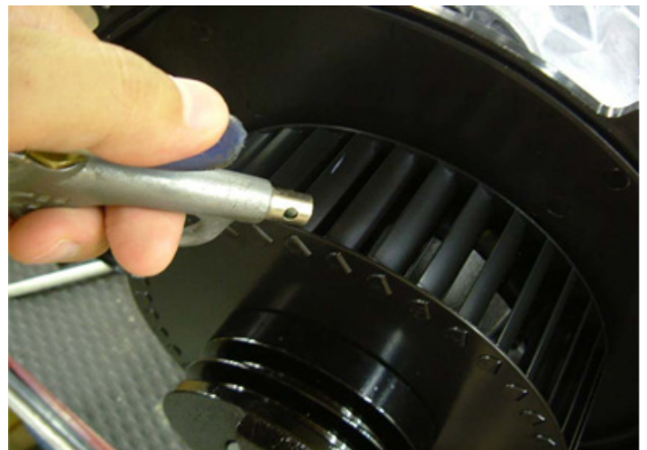
Figure 56: Using compressed air to remove dust from the cooling fan.
