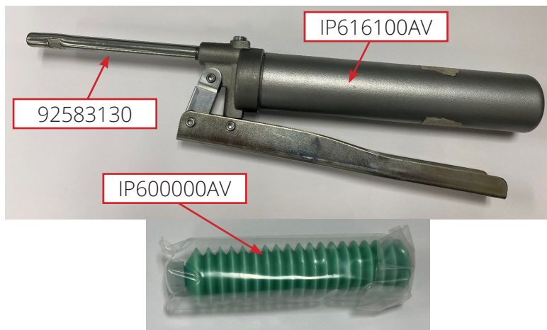
Figure 21: Grease, grease gun, and nozzle required
