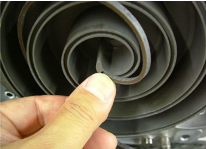
Figure 38: Begin insertion of the HP Tip Seal at the center of the scroll.
