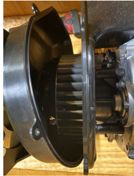
Figure 55: Fan Shroud opened for cleaning
