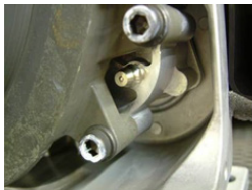
Figure 30: Pin Crank Bearing Grease Fittings
