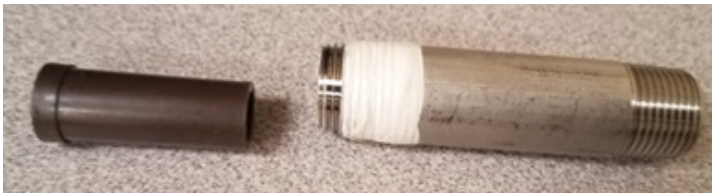
Figure 50: Insulation tube on the left.
