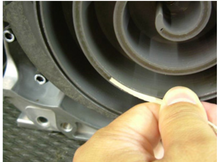
Figure 40: Butt the LP Tip Seal up against the HP Tip Seal. Be sure the lip seal tips are pointed in the correct direction.
