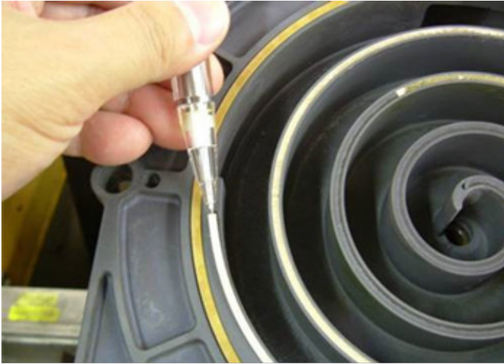
Figure 32: LP Tip Seal Removal
