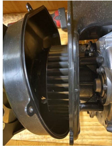
Figure 55: Fan Shroud opened for cleaning
