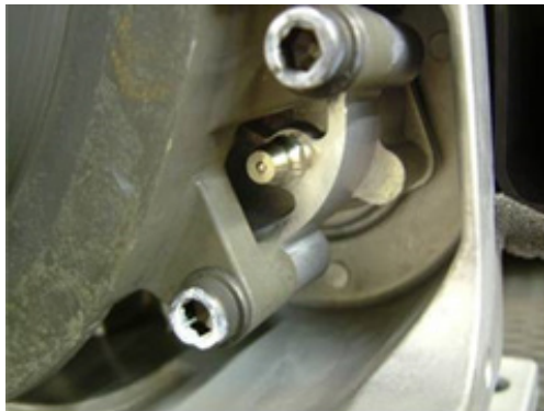
Figure 30: Pin Crank Bearing Grease Fittings
