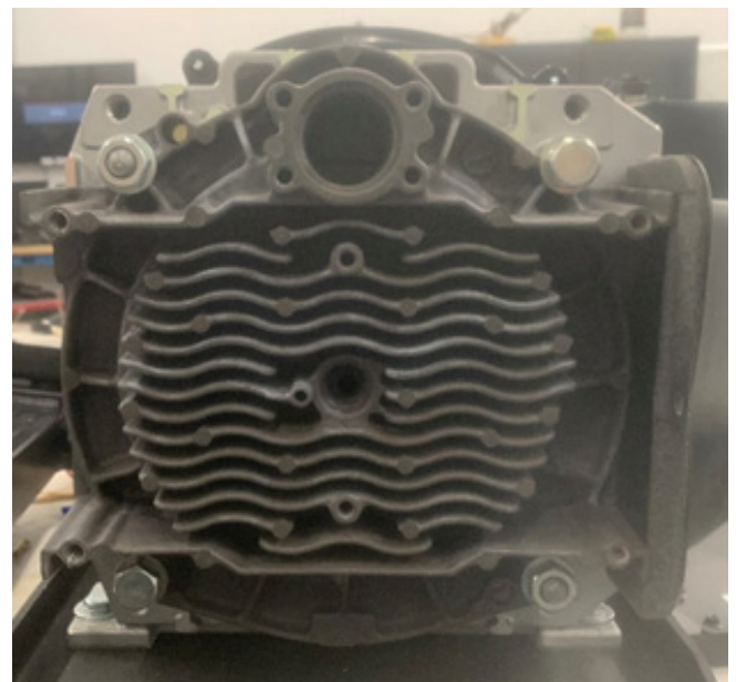
Figure 52: Fixed scroll with fins exposed
