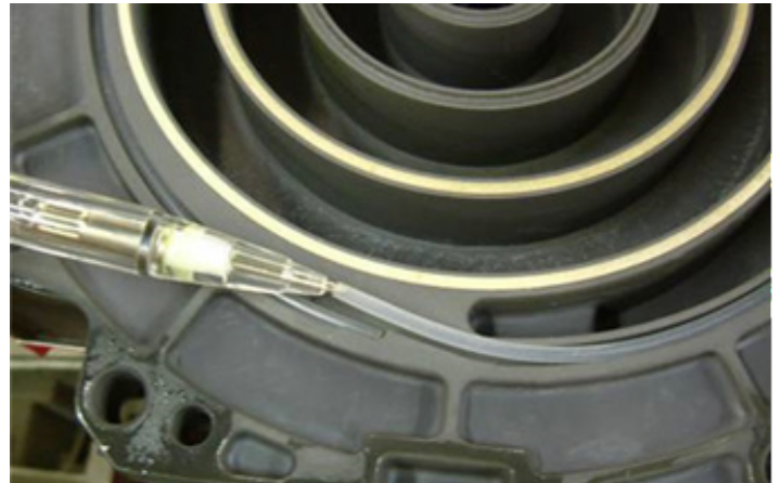
Figure 35: Back-up Tube Removal
