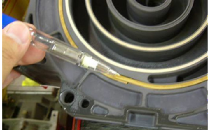
Figure 34: Dust Seal Removal
