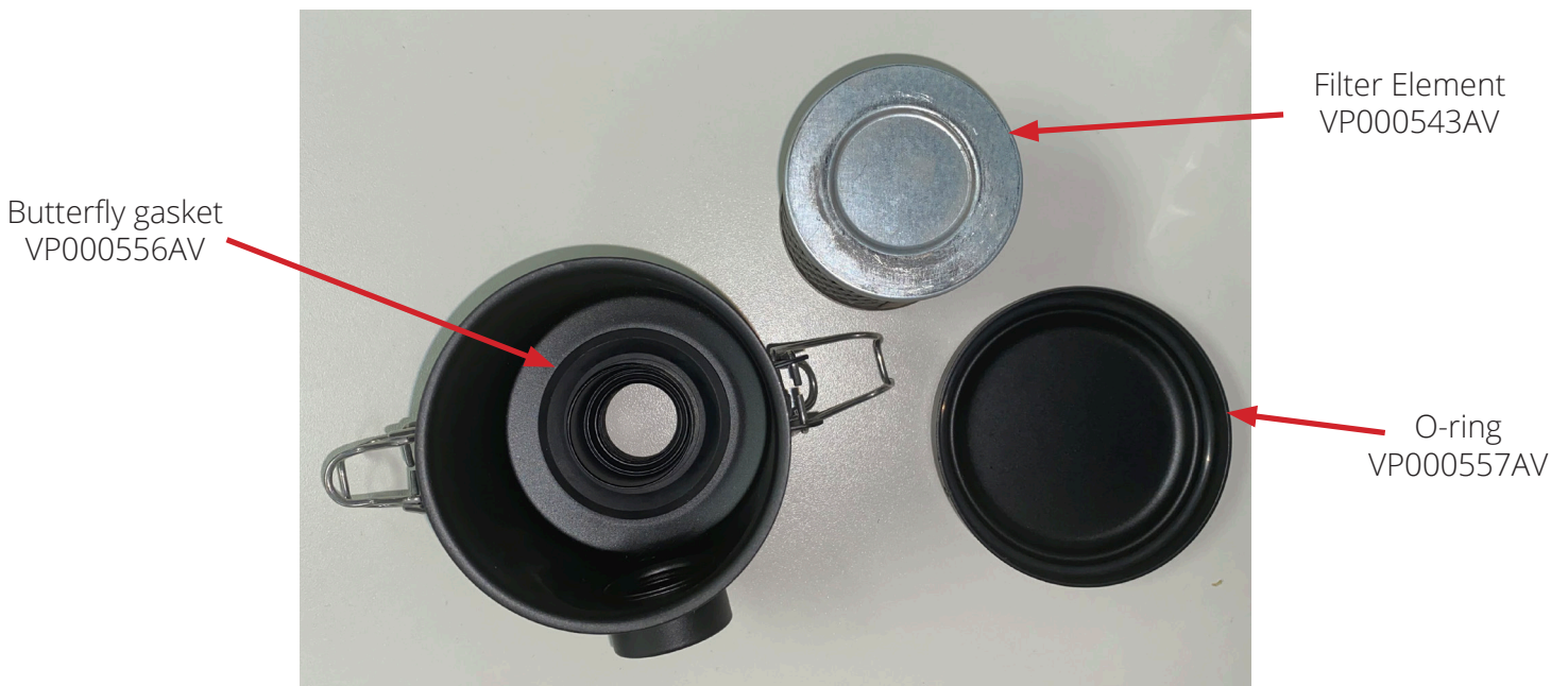
Figure 59: Serviceable parts for VP000542A. The highlighted parts come with the VP000558AJ service kit.
