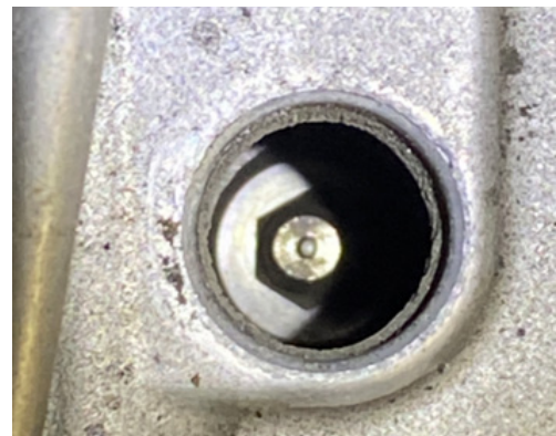
Figure 24: View of the grease fitting through the grease access hole when rotated into the correct position for greasing
