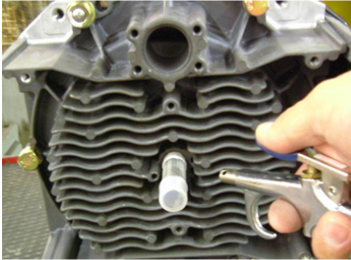
Figure 53 : Using compressed air to remove debris from the fins.
