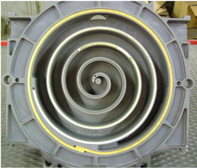
Figure 95: Install dust seal on top of the back-up tube.
