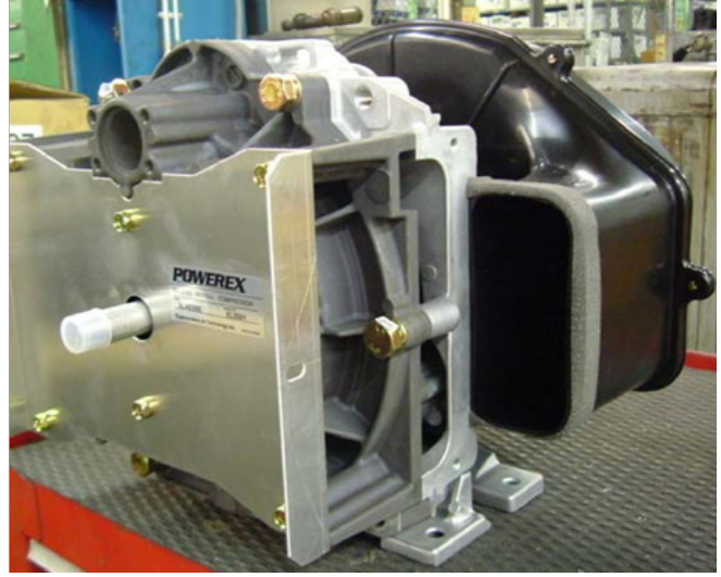
Figure 77: Air end with Fan Duct removed
