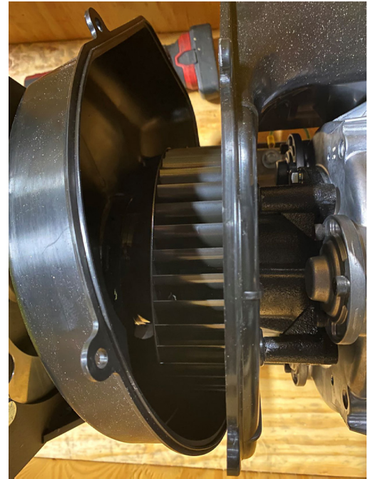
Figure 104: Fan Shroud opened for cleaning
