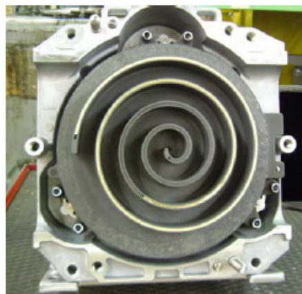
Figure 85: OS. OS acts as mating surface for the dust seal in the FS. The OS does not contain a dust seal
