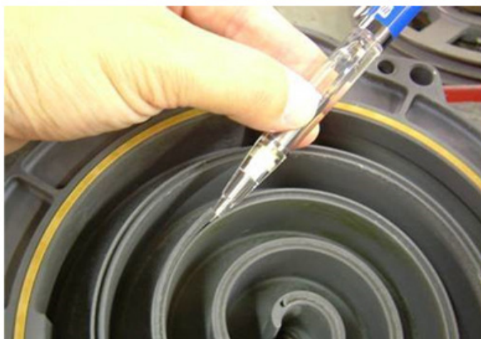
Figure 82: HP Tip Seal Removal
