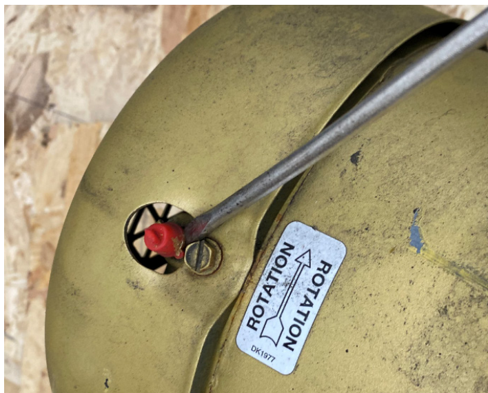
Figure 128: Use Flathead Screwdriver to remove Protective Caps
