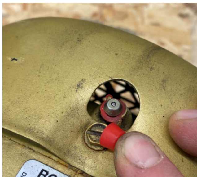
Figure 129: Grease Fitting Uncovered
