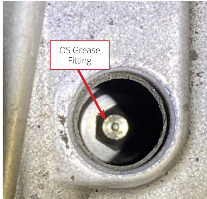
Figure 73: View of the grease fitting through the grease access hole when rotated into the correct position for greasing
