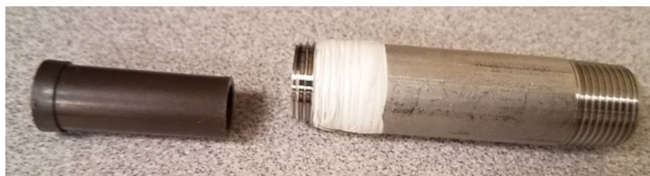
Figure 99: Insulation tube on the left
