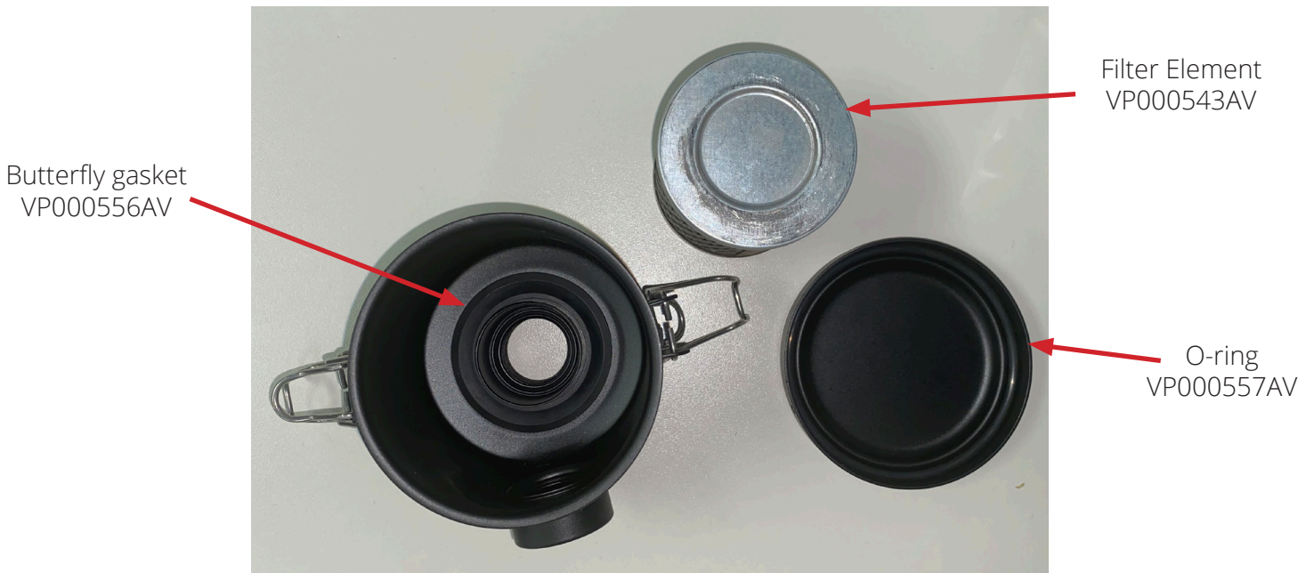
Figure 120: Serviceable parts for VP000542A. The highlighted parts come with the VP000558AJ service kit.
