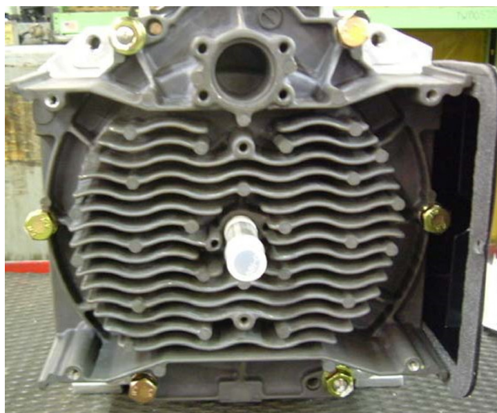
Figure 101: Fixed Scroll with cover removed
