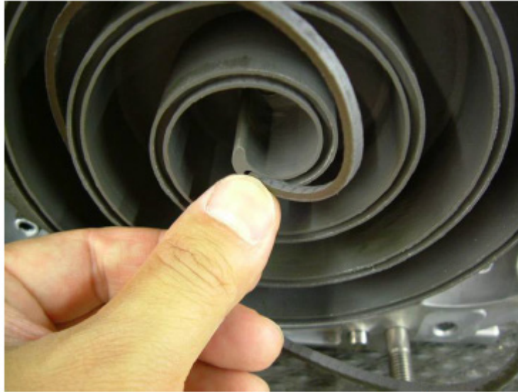
Figure 87: Begin insertion of the HP Tip Seal at the center of the scroll.
