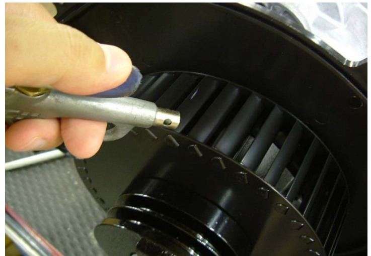
Figure 105: Using compressed air to remove dust from the cooling fan.
