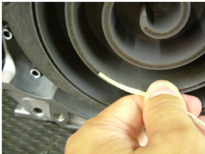
Figure 89: Butt the LP Tip Seal up against the HP Tip Seal. Be sure the lip seal tips are pointed in the correct direction
