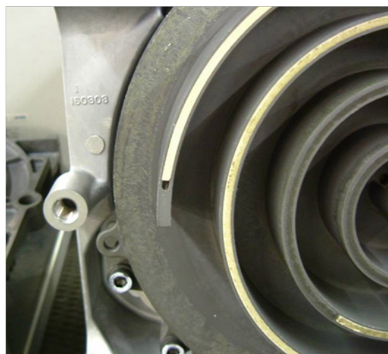
Figure 93: Seat the trimmed seal.
