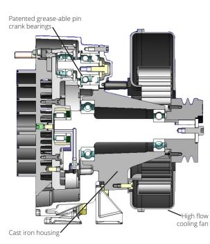
Our innovative scroll technology is completely oilless, extremely quiet, and energy efficient. The scroll pump has few moving parts, making it reliable and easier to maintain. The self lubricating tip seals and absence of a gearbox means the pump is truly 100% oil free. As leaders in scroll pump technology, our design incorporates several innovative features:
